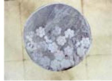
Fig. 3: Properly grouted tendon section
